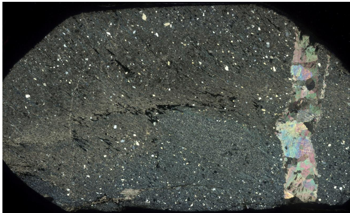
Sample 863680. Wide-field, full-thinsection view showing mylonitic schist with four mineralogical domains and calcite vein. Top- plane light; Bottom- crossed polarizers.
