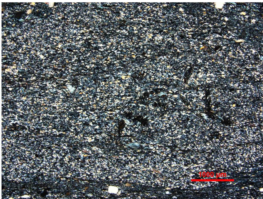
Sample 863680. Very quartz-rich, quartz-chlorite-ilmenite assemblage in Domain III. Note lack of relict quartz grains in this domain. Top- plane light; Bottom- crossed polarized.
