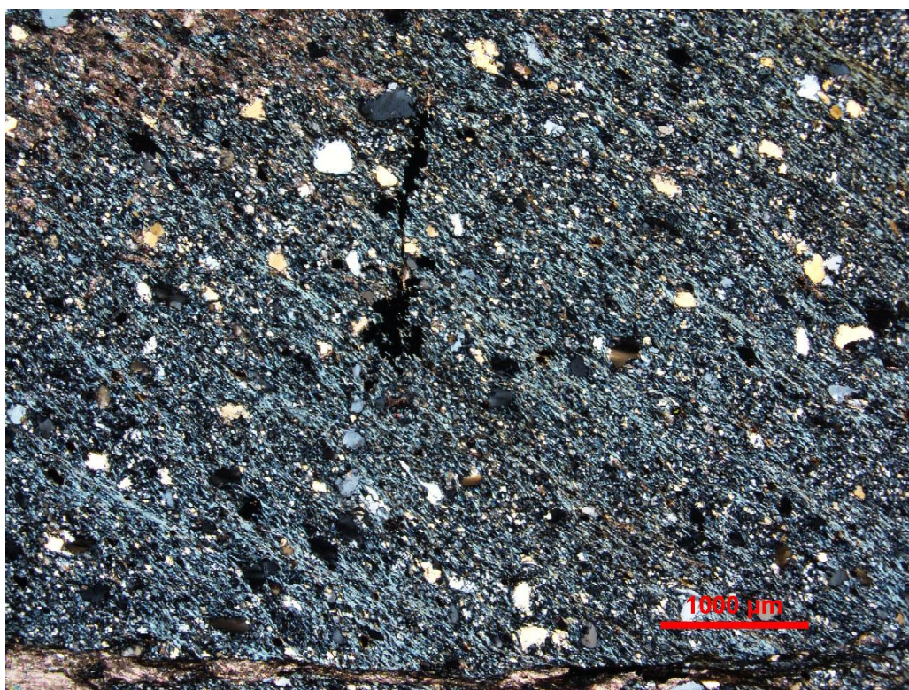
Sample 863680. Domain II with very abundant chlorite, minor carbonate and relict quartz grains in moderate-strong foliated mylonitic schist. Note contact with Domain I in upper left corner. Top- plane light; Bottom- crossed polarizers
